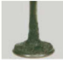
Intake valve before P.i. treatment.
