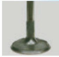
Intake valve after P.i. treatment.
